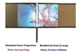
When comparing both "RP" and "Dual" materials projecting from the rear and viewing from the rear—The "RP" material is ill suited to perform well when viewed from the same angle of projection. Notice the hot spotting and "cold-spots" on the RP, while the Dual material provides the same brightness and uniformity as seen in the previous photo comparison.
